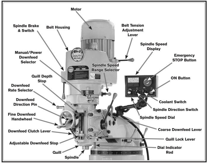
Figure 2. SB1027 drive system and headstock identification.
